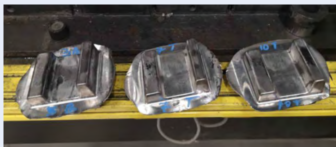
Figure 2: As-forged magnesium parts (Courtesy University of Waterloo)
