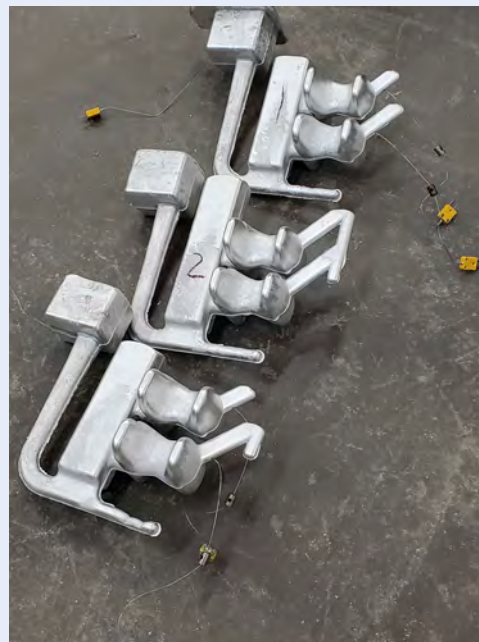
Figure 1: Re-cast magnesium pre-forms (Courtesy University of Waterloo)
