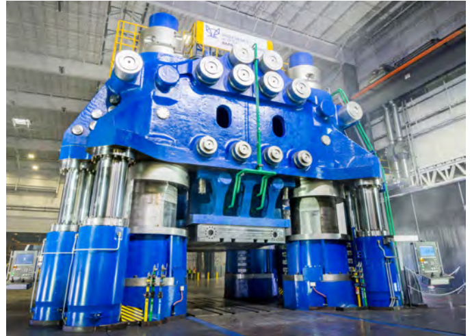
Weber Metals' massive 60,000-ton press is used to produce larger forgings of aluminum and titanium (Courtesy of Weber Metals)
